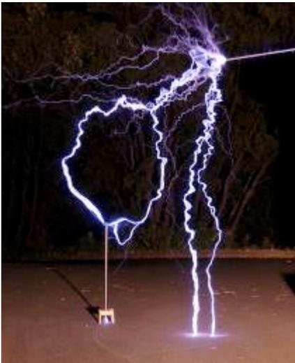
**Picture 1.** Shows Mulpin PCB being subjected to the high voltage of the Tesla Coil. Note the spark jumping to ground just under the stand holding the PCB. The spark to ground is about 2 metres long.
