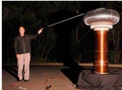
**Picture 2** shows Tesla coil alongside the Lead Inventor for scale. He is 1.85 M tall.
